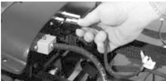
Figure 18. Disconnecting The Battery Harnesses
